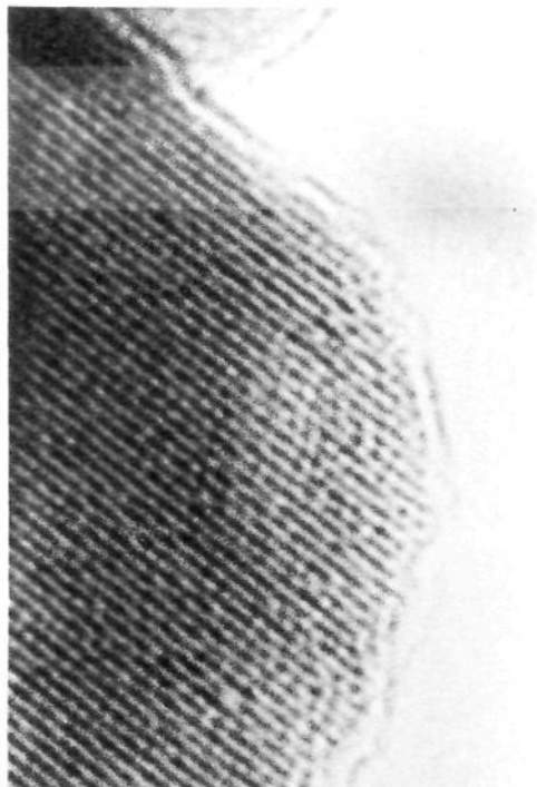
Figure 5. High-resolution transmission electron micrograph lattice image of 12[WO 3 ]-Na 56 Y.
